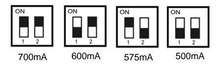
The driver will be shipped out of factory with both switches set to ON (700mA).
